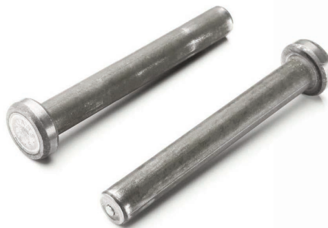
Cheese head, flux charge, and shank - the three key functional zones of a shear connector
